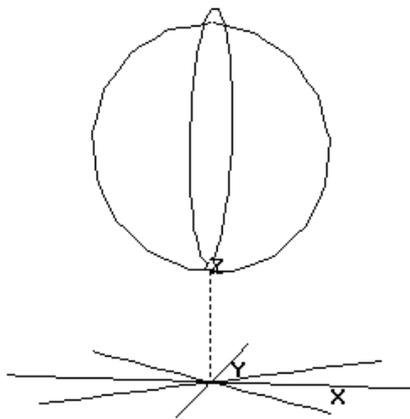
**VHF Eggbeater Calculation:** - Copper 2-mm diam. (0.08 in) was used for preliminary test.
