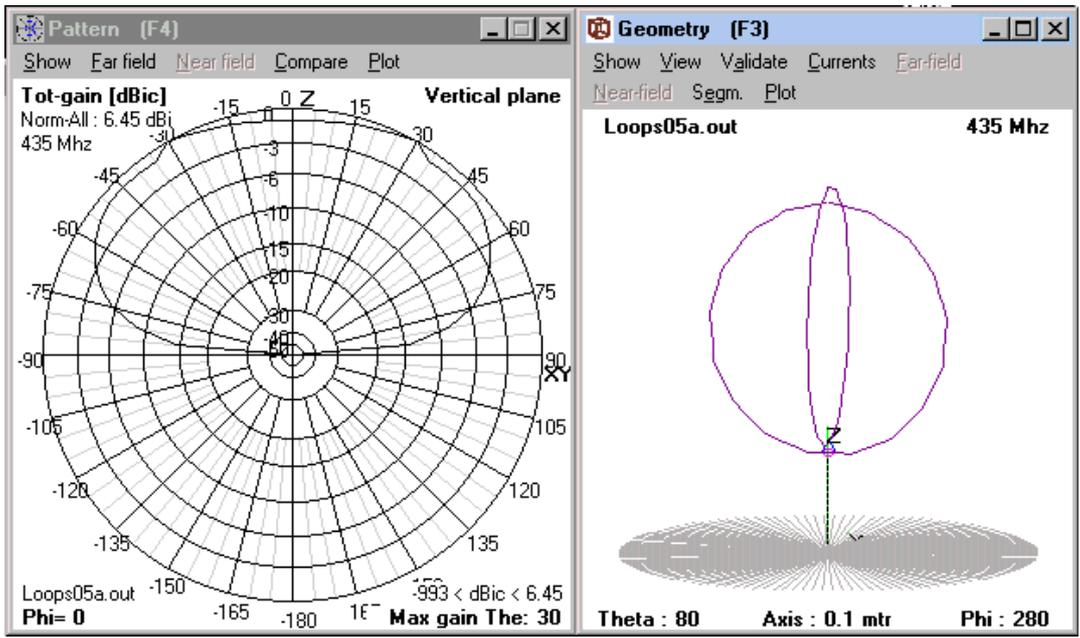
Fig 1 'Eggbeater' over a perfect ground reflector (spacing is 1/8 wavelength)
