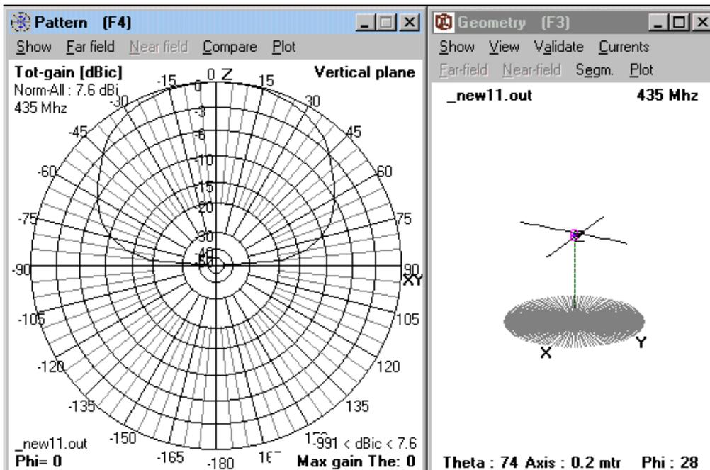
Fig 3 ' Turnstile ' antenna over a perfect ground reflector.
