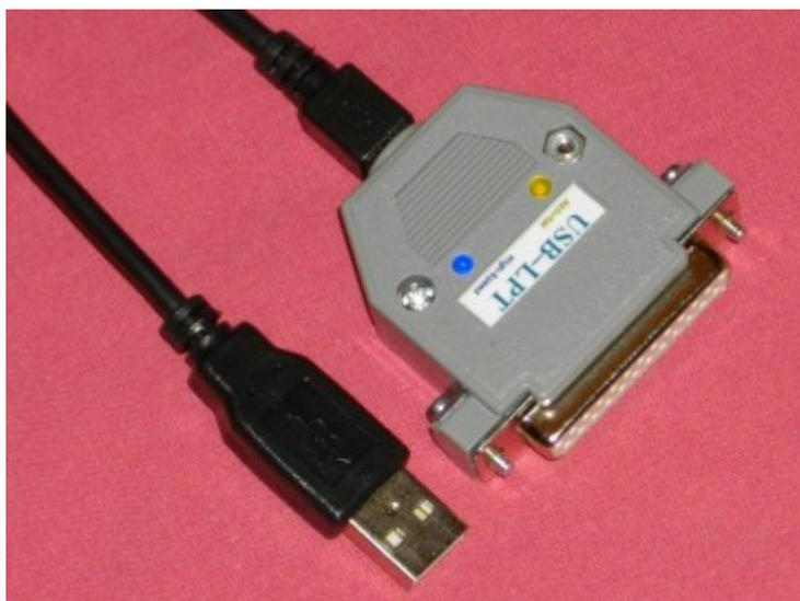
**Fig 2 USB / PARALLEL Converter USB2LPT 1.7**
