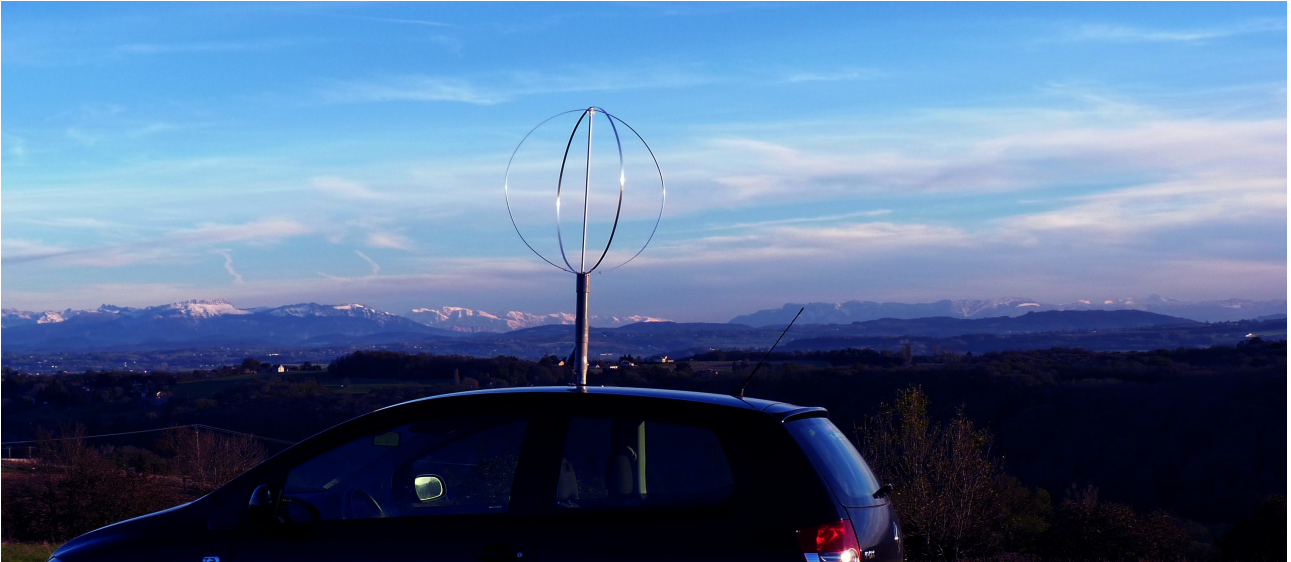
~ “Eggbeater Antenna” used in mobile traffic ~
